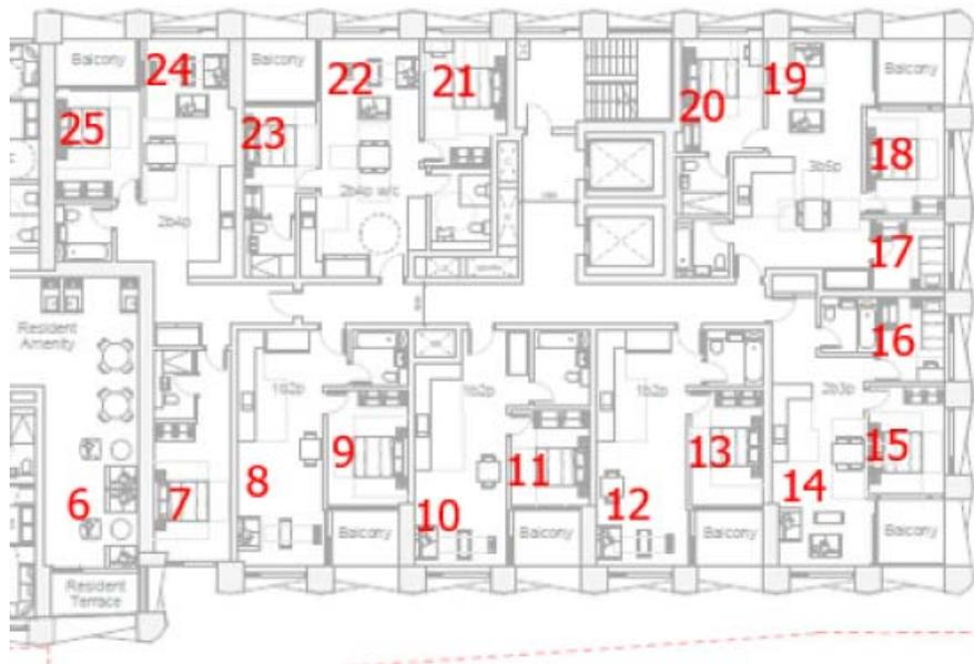
Image 10: C3 layout and rooms tested for daylight levels
