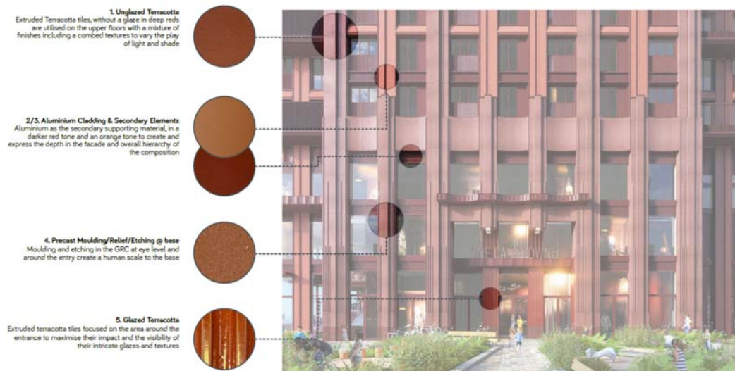
Figure 32: Materiality of Building A
