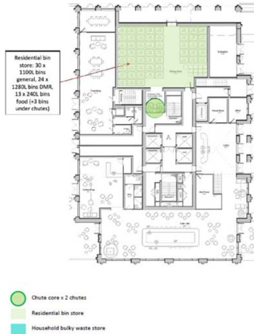
Figure 71- Layout of bin stores for Building B
