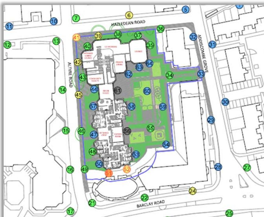
Figure 59: Wind speeds at ground level, prior to amendments
