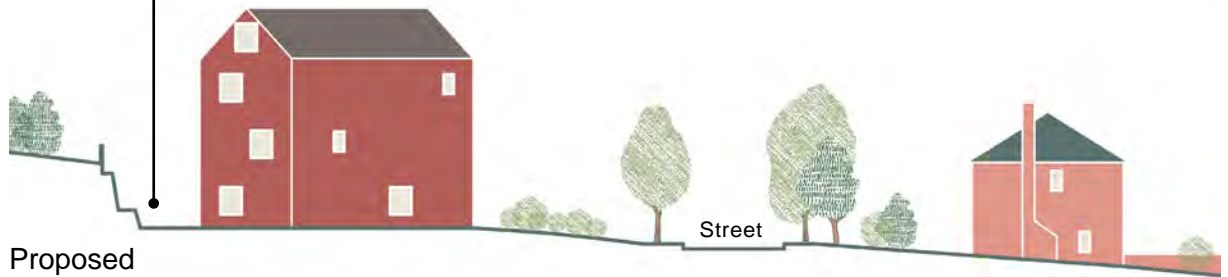
Figure 2.20b: A proposal for redevelopment with semi-submerged ground floor, including lightwell to rear, making use of the topography to provide additional accommodation.
