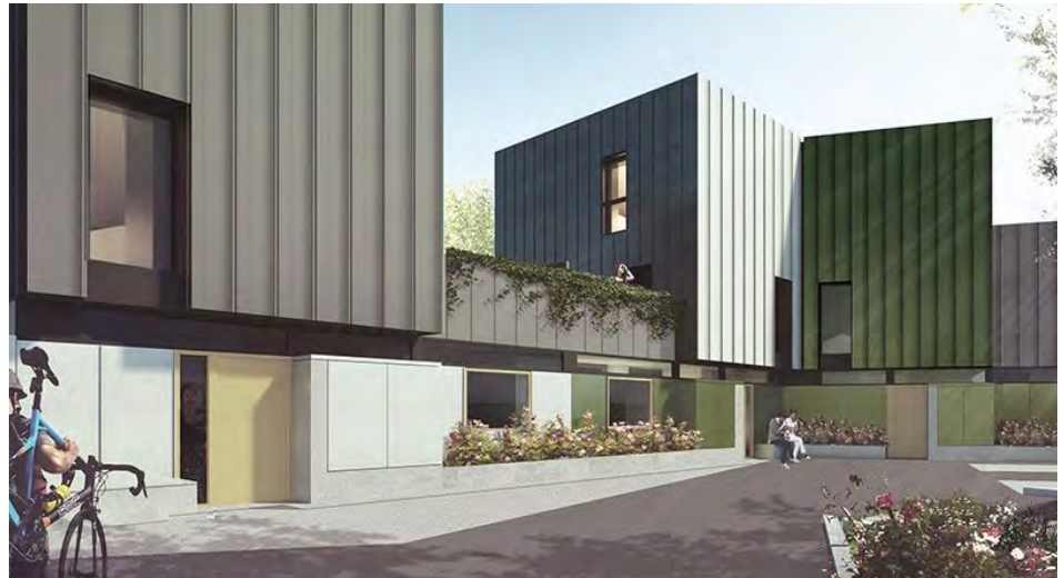
Figure 2.13b: Visual of a proposal for a back land development by Coffey Architects where the height has been stepped to maintain sense of openness.
